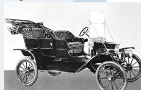
Ford Model T, combustion engine, 20 HP, in 1910
