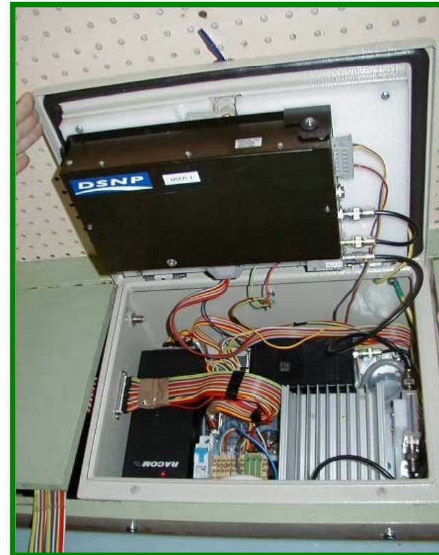
GNSS/ INS based train position locator in the locomotive cabin.
